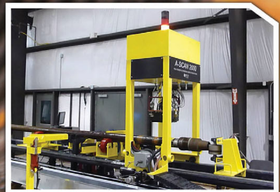
ASCAN 2000 Full Length Ultrasonic Inspection
