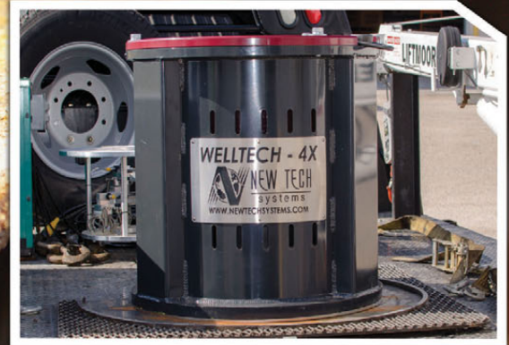
WellTech 4X EMI Inspection for Tubing On Rig Floor
